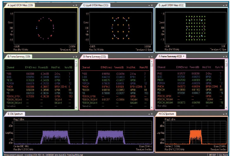
Figure 2: Agilent 89600 VSA software acquires the inter-band signal from two signal analyzers and analyzes all CCs simultaneously.
